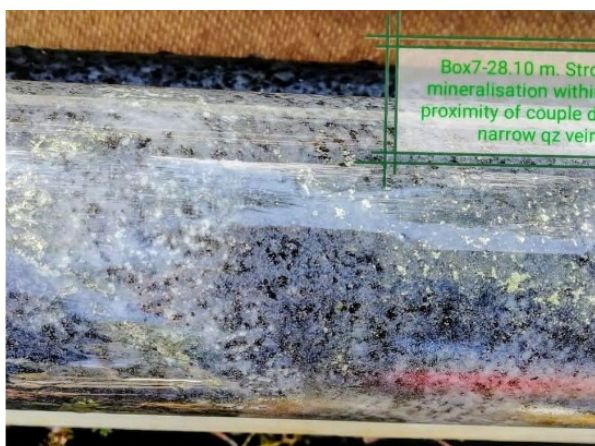
Figure 4. Core from the 2021 Isoneva Drill Program Showing Strong Sulfide Mineralization; Assays Pending
