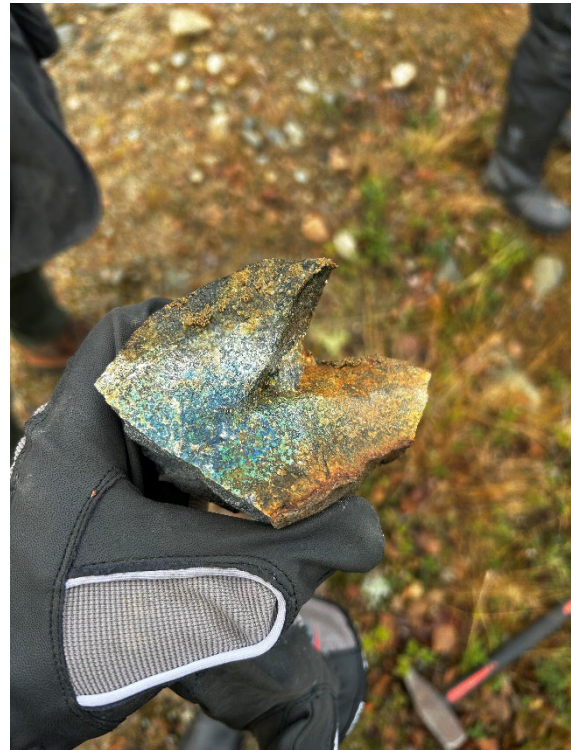
Figure 1 Rock Sample from Boulder on Paksuselka License showing Abundant Copper Oxide Mineralization
